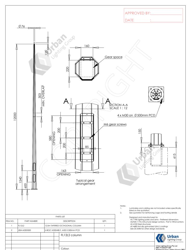
Luminaires allowed for: 1.2 sq.m 120kg total load
