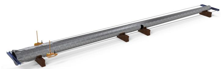
Set up 2 winches on either side of the column, with beams across the ends so that the winches will pull the column sections together evenly.
