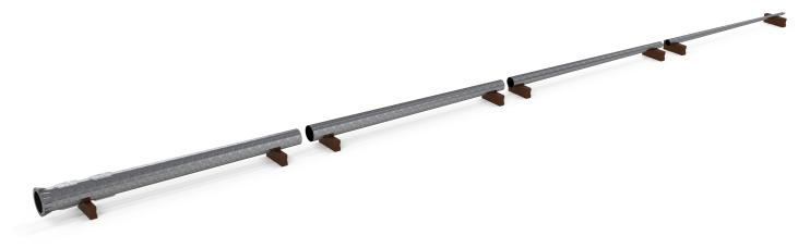
Arrange the column sections from the base to the tip, with bearers under the end of each section. If the ground is not level, you may need to add bearers to get the sections into a straight line. Make sure that the bearers are clear of the joints.
